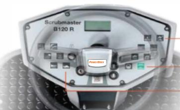
The boost button activates both maximum brush pressure and water flow.
